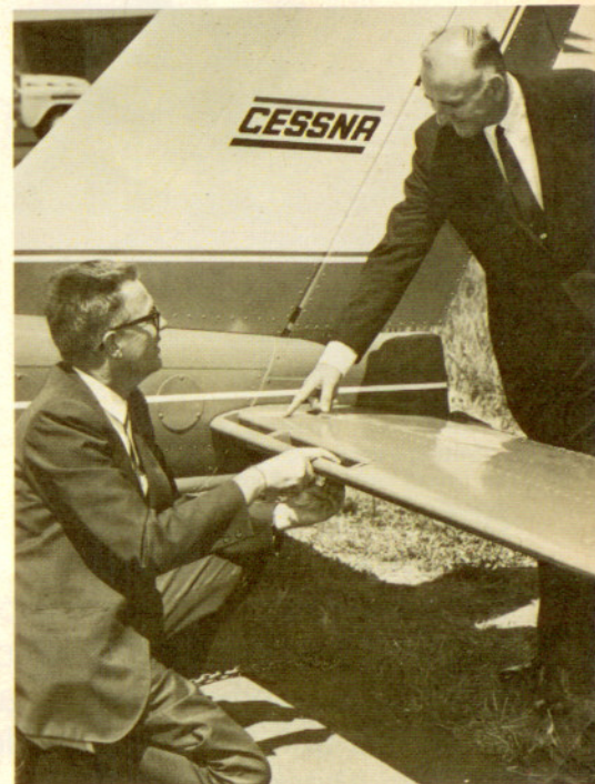
Cessna's W.D. Thompson points out to Don Downie the stabilator fix given a Cardinal under the company's Cardinal modification program.
